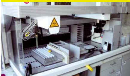
Figure 1a: Tecan GENESIS 150 workstation. The workstation is an open source system and can also be used now for kinetic samples. It has an integrated Sunrise™ spectrophotometer and uses TOPS™ 4.0 with Magellan
